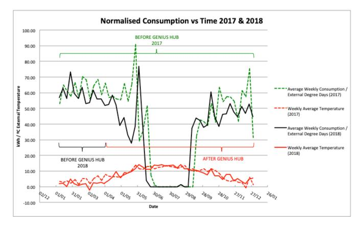
Figure 6 – Normalised consumption vs Time (2017 & 2018) (Figures 2 & 5 augmented).
