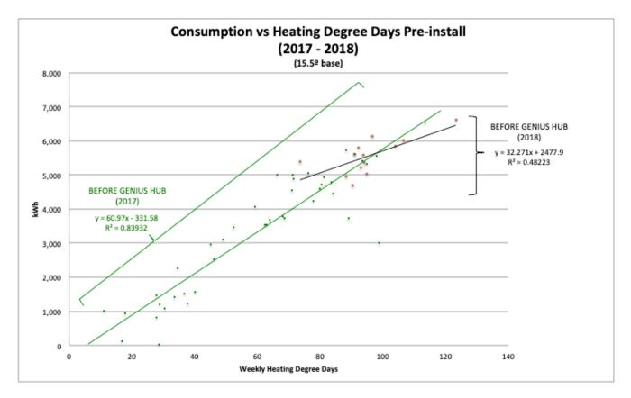
**Figure 3** – Graph showing energy consumption per weekly heating degree days prior to installation of Genius Hub system (01/01/2017 -> 31/03/2018).
