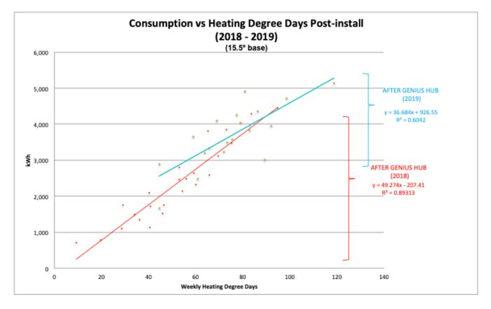
**Figure 7** – Graph showing energy consumption per weekly heating degree days after installation of the Genius Hub system (01/04/2018 -> 01/05/2019).
